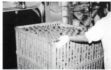
Screens available in various hole sizes. The seamless all-plastic retort separator is made from tough, durable polypropylene, which is heat and corrosion resistant. Long hours of trouble free service will reduce operating costs in food processing.
